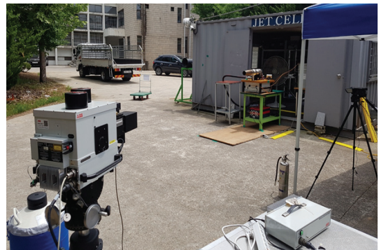
Fig. 1 Engine Plume IR Signal measurement.
