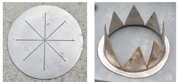
Fig. 9. Diaphragm(left: before test, right: after test)
