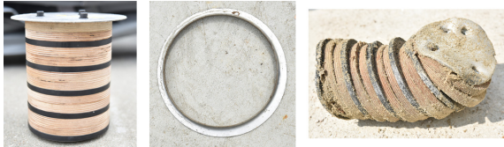
Fig. 10. Piston(before test), shear ring, piston recovered(after test)
