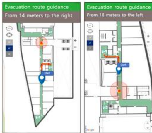
Fig. 4. Guidance of evacuation routes using the navigation app on the smartphone
