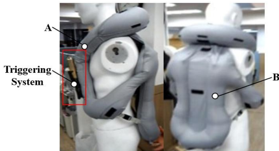
Fig. 5 Photograph of airbag system
