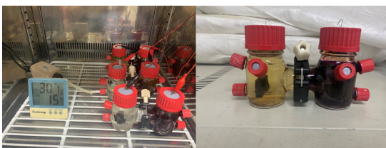
Fig. 2. Dual chambered microbial fuel cells
