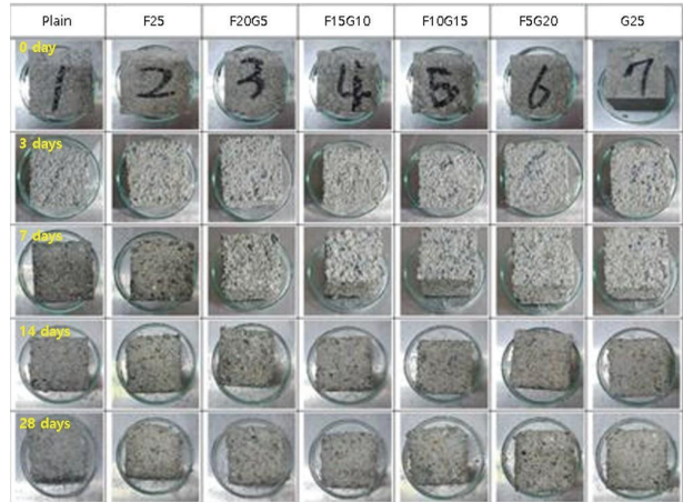
Fig. 6. Sulfuric acid resistance test
