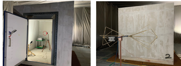
Fig. 5. SE test environment of concrete block
