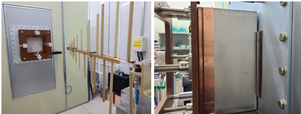
Fig. 3. SE test environment of concrete block
