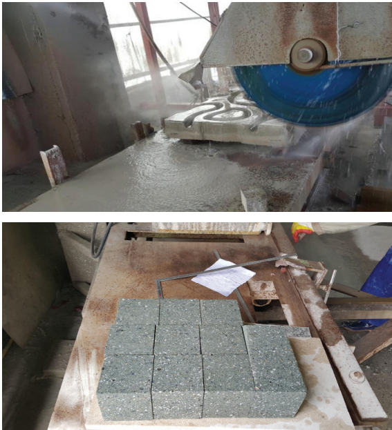
Fig. 2. Concrete block test body
