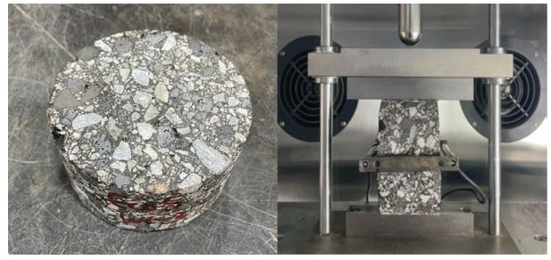
Fig. 3. Test equipment and testing materials of fatigue crack
