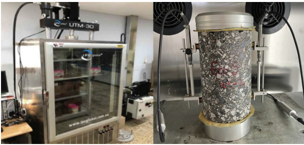
Fig. 2. Test equipment and testing materials of dynamic modulus
