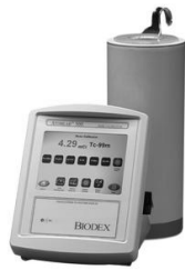
Fig. 3. When using the dose calibrator, the radioactivity source was set to a volume of 0.1 ml in a 1 cc type syringe, placed in a dedicated sample holder, and then radioactivity was measured.
