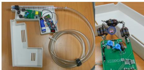
Fig. 15. Plasma generation prototype with PZT devices
