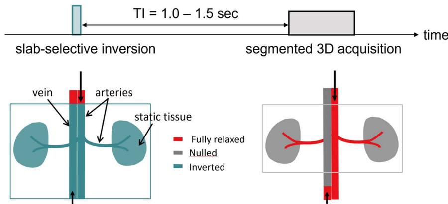
**Fig. 5.** Principle of slab-selective inversion recovery angiography. The pulse sequence consists of slab-selective inversion, delay time of 1.0-1.5 sec, and segmented 3D acquisition. During the delay time, inverted static tissues and venous blood can only recover partially whereas upstream arterial blood is not affected by the inversion pulse flow into the imaging volume, thereby exhibiting high signals in resultant images.
