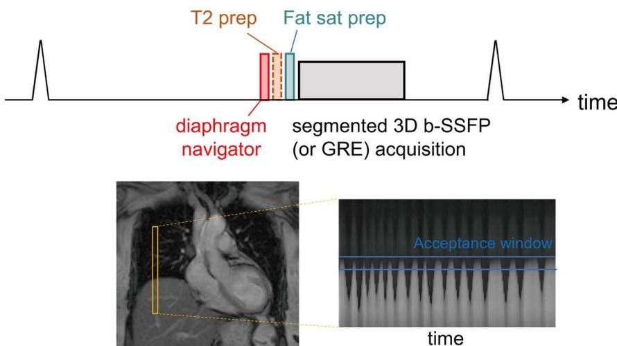
**Fig. 7.** Principle of free-breathing 3D coronary angiography. The pulse sequence is cardiac gated. It applies respiratory navigator, T2 preparation, fat saturation, and segmented 3D acquisition. The respiratory navigator applies pencil beam-shaped excitation across the liver-air interface to obtain 1D signals over cardiac cycles. It decides whether to record or abandon data segments obtained in the same cardiac cycle based on a pre-defined acceptance window.
