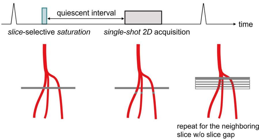
**Fig. 6.** Principle of quiescent interval single-shot imaging (QISS). The pulse sequence consists of thin saturation preparation, quiescent interval period, and single-shot 2D acquisition. During the quiescent interval, saturated static tissues recover only partially while fresh upstream arterial blood flows into the imaging volume. This is repeated multiple times for neighboring slices without a slice gap to form 3D volume of angiogram.
