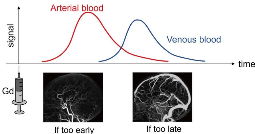
**Fig. 2.** Time-signal curves for arterial blood and venous blood in gadolinium-based contrast enhanced MR angiography. As the contrast agent flows through the vascular system, arterial blood and venous blood light up sequentially due to increased T1 values by the contrast agent. Image captured too early after the injection of contrast agent may fail to depict distal arteries, while images captured too late may suffer from venous contamination.
