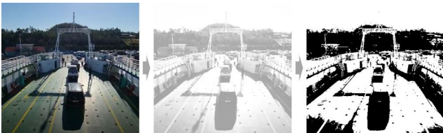
Fig. 5. Vehicle detection result through difference image.
