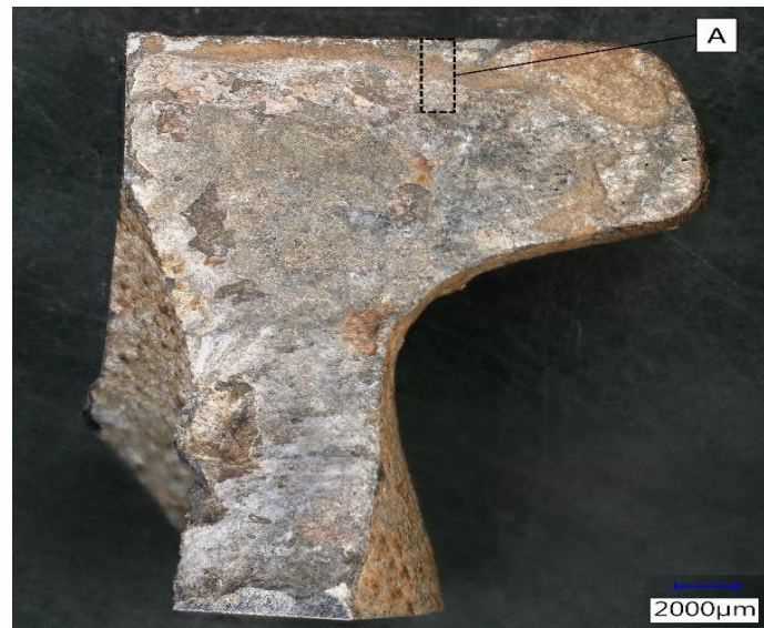
Fig. 2. Fracture surface obtained by digital microscope
