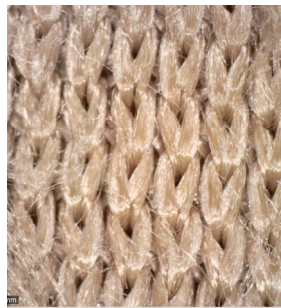
(b) Digital Microscope image of based fabric (×60)
