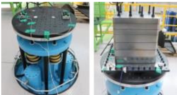
Fig. 4. LVSM test setup w/o payload(left) and payload 500 kg(right)
