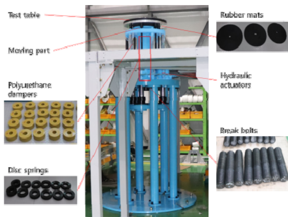
Fig. 1. Structure and main components of LVSM
