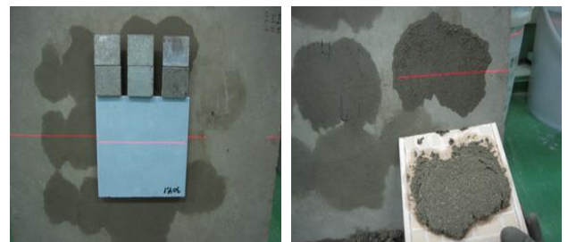
(a) loading after tile direct setting (b) tile removing
