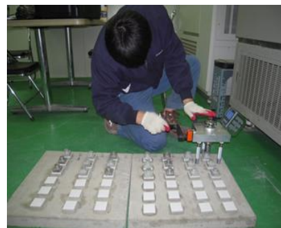
Figure 4. Adhesive strength test
