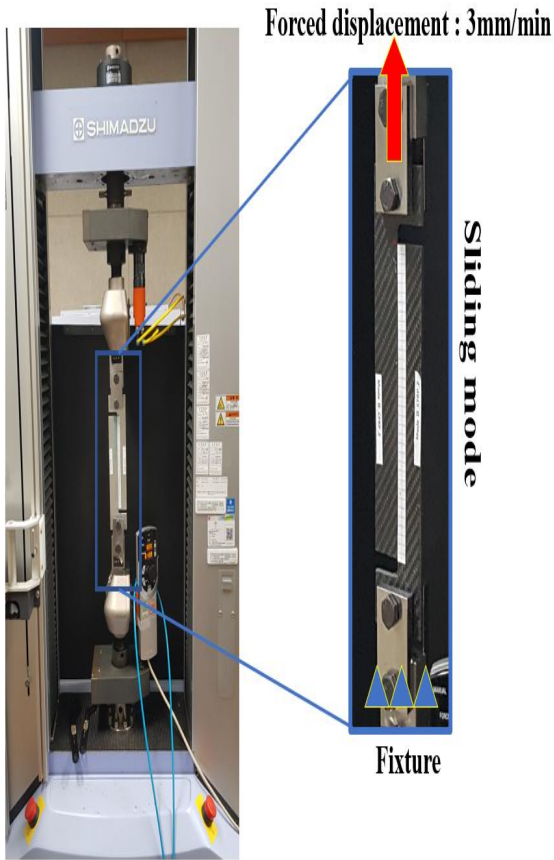
Fig. 5 Specimen held for mode II and the experimental condition
