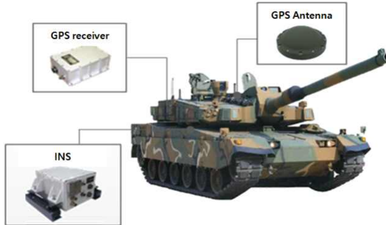
Fig. 1. Position of the hybrid navigation system on combat vehicle
