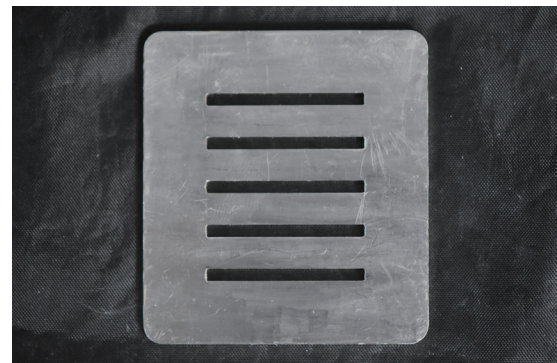
Fig. 1. Stainless steel mold mold to fabricate temporary restorative resin specimens by conventional method (45 x 50 x 2 mm)
