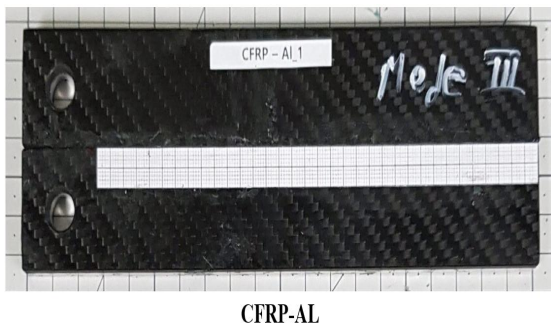
Fig. 14 Shape of double cantilever beam specimen with heterogeneous materials(CFRP-AL)
