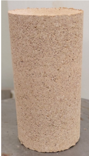
Fig. 5. Ze-EICP specimen for unconfined compression test
