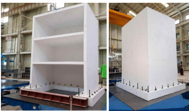
Fig. 1. Reinforced concrete building anchored onto shake table
