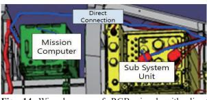
Fig. 14 Wire harness of RGB signal with direct connection.
