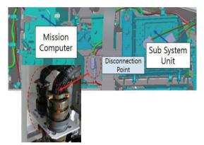
Fig. 7 Video signal path between the sub system and the mission computer.
