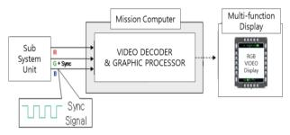
Fig. 6 RGB and Sync signal from sub-system.
