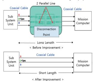
Fig. 13 Improvement in cable configuration.
