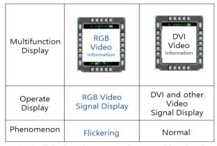
Fig. 2 Flickering phenomenon in RGB video signal.
