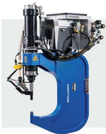
Fig. 3 C-Frame for SPR joining process [3]
