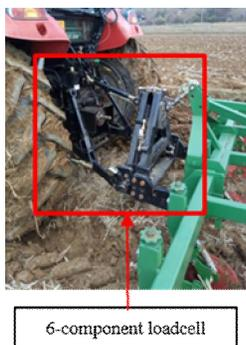
**Fig. 2 6-component loadcell mounted on the tractor**
