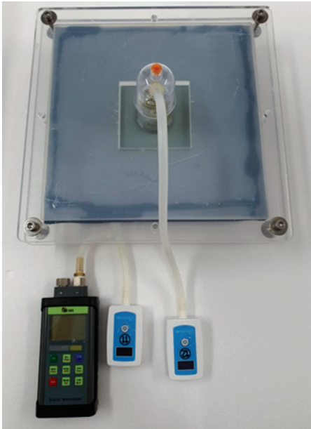
Fig. 2. Skin model with digital manometer and layer cupping with 2 Dongbang cups.
