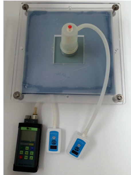
Fig. 3. Skin model with digital manometer and layer cupping with a Dongbang cup and a cup made by 3D printing.
