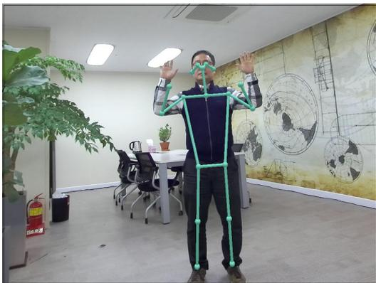
Fig. 6. Result of Motion capture using Pose Estimation
