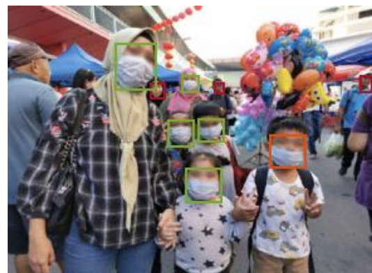
Fig. 9. Mask detection result using our proposed system (green: with mask, orange: Mask worned incorrectly, red: without mask)
