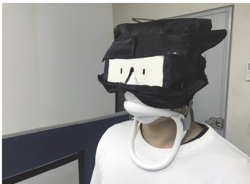
Fig. 4. Picture of wearing glasses that limits field of view and neck supporter that limits head movement in real environment
