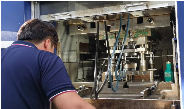
Fig. 5 Try out of fine blanking trial mold
