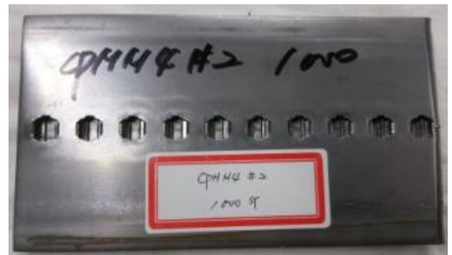
Fig. 13 Strip layout of pocket punch in the fine blanking trial mold
