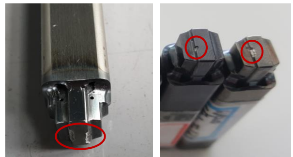
Fig. 15 Damaged pocket punch in the fine blanking trial mold
