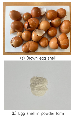
Fig 1. Eggshell processed to be used as a shielding material
