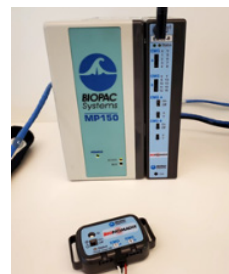
[Fig. 2] EMG measurement setup (Biopac MP150 with a wireless EMG module)
