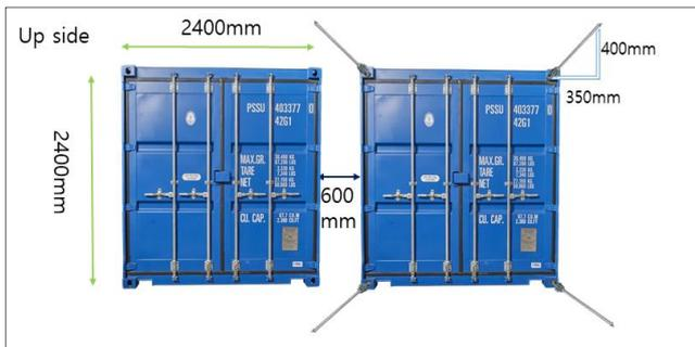
Fig. 2. 10ft container stowage deployment.
