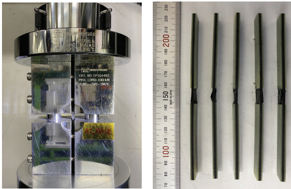
Fig. 6. Setup for no hole laminate compression test and specimens after failure
