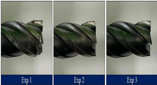
Fig. 16 Cutting tool condition
