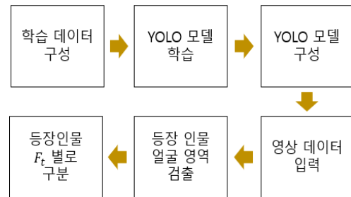
Fig. 3. Work Steps of Face Estimation Data F_t :Frame(F) over Time(t)
