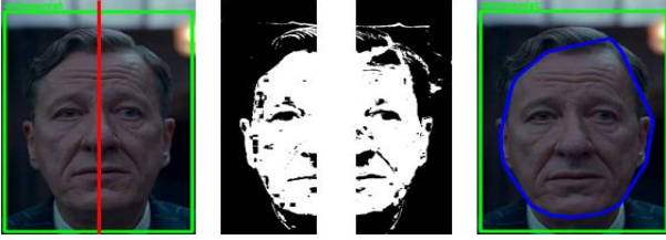
Fig. 11. Steps of Face Contour Detection Using Split Rectangle (Antagonist)
