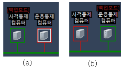
Fig. 17. Self-reconfiguration results of controller-failure scenarios (a) failure of controller (Case 1) (b) failure of controller(Case 2)
