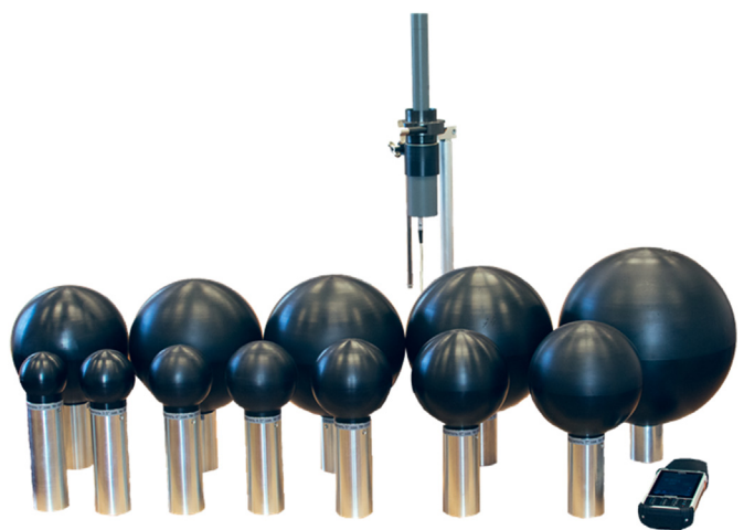
Fig. 3. AT1117 M spectrometer with the BDKN-06 unit and the set of spheres.
