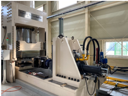
Fig. 4 Dynamic test machine for base isolation systems
