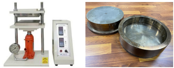
Fig. 2 Hot-press and mold to prepare sample in this study
