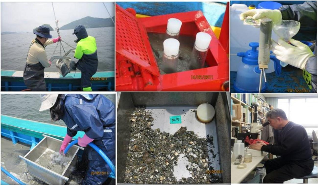
Fig. 1. Photographs showing the procedures for producing the quantitative biological data on macro- and meiozoobenthic samples in coastal areas from sample collection in the fields and sieving and species identification in laboratories.
