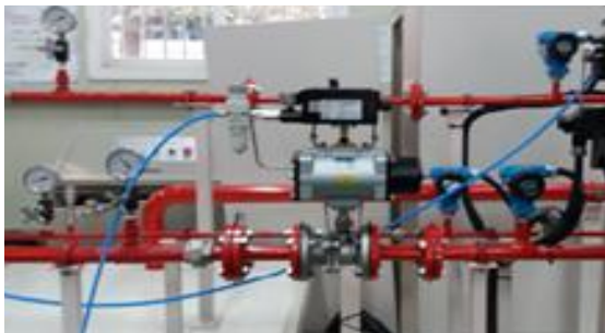
Fig. 3 Experiment setup for 1-inch control ball valve
