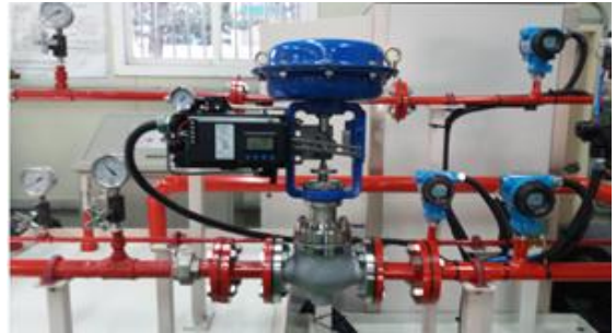
Fig. 4 Experiment setup for 1-inch control globe valve
