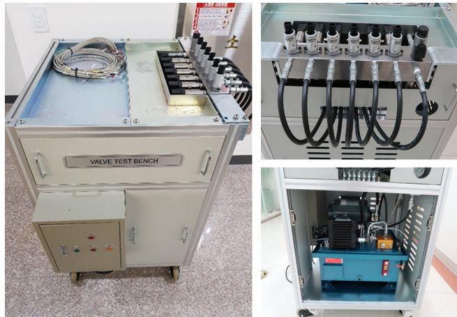
Fig. 3. Photos of test bench for stability evaluation of proportional valve controller.
