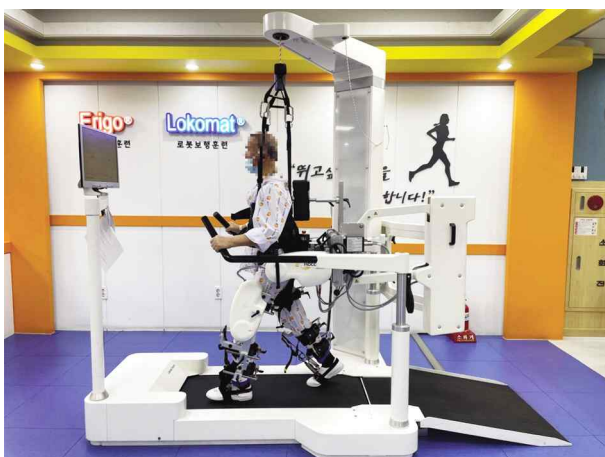
Figure 2. Robot assisted gait training using the Lokomat®
