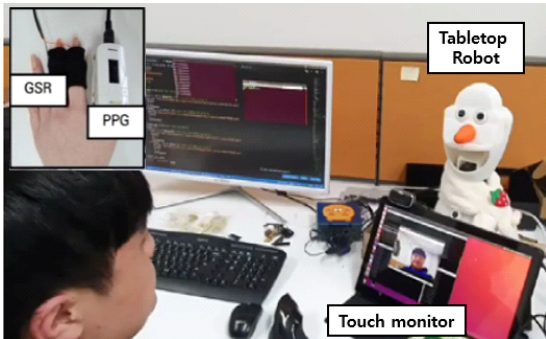
Fig. 7 Experimental setup for estimating the user's psychological state using a robot
