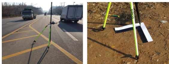
Fig. 3. Control point survey by GNSS
