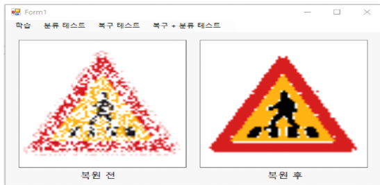
Fig. 3 Restoration of traffic signs using Hopfield Network
