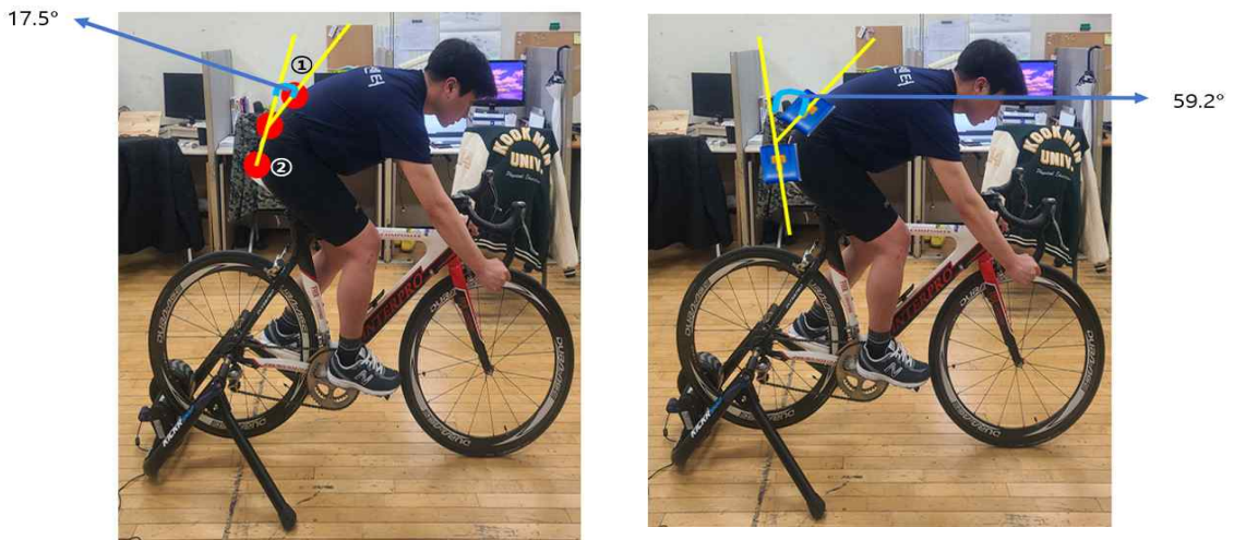
Figure 8. Lumbar Flexion Angle 30° 3D Motion Capture System(17.5°) VS IMU Sensor (59.2°) (taken by authors)
