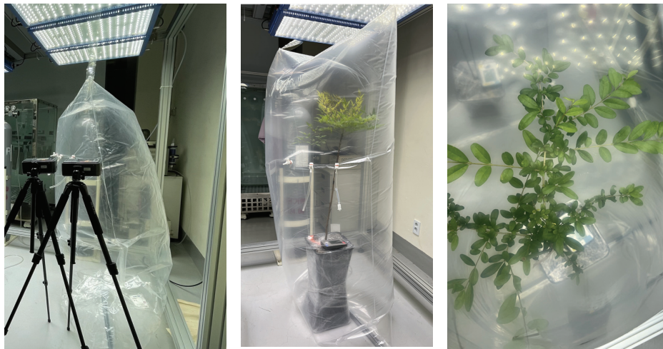
Figure 1. Chamber system for BVOCs sampling.
