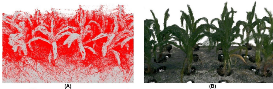
Fig. 4. Result of statistical outlier removal for point cloud data. Red points and gray points indicate noise and inliers, respectively. (A) Point cloud data of sorghum before statistical outlier removal (SOR) (B) sorghum data after SOR.
